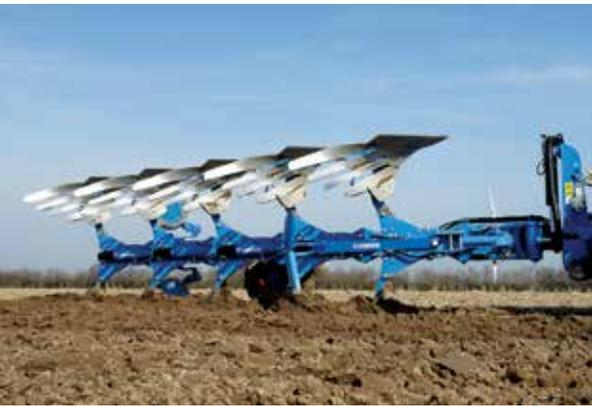
I plough a lot in the summer to turn the soil upside down and dry out weed roots, but my heavy clay soil dries out fast, creating lumps that are hard to break up. My JUWEL plough with VARIOPACK has made the job easier and more efficient because as I plough, the packer breaks up lumps and removes air pockets which can settle after seeding and disturb plant roots. I get a solid, smooth seedbed in one pass and have more even plant stands.
