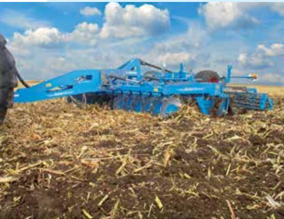
The RUBIN 12 compact disc harrow was designed to handle large volumes of crop residue from the highest yielding corn crops in North America. The RUBIN 12's 29-inch, concave discs work deeper to incorporate heavy residue and create a smooth seedbed that's ready to go with a single pass.
