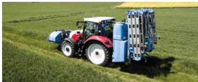
The front tank is particularly advantageous on narrow tracks or in hilly environments, as it makes for a compact system that is much more agile than comparable trailed field sprayers, despite the large tank volume.
