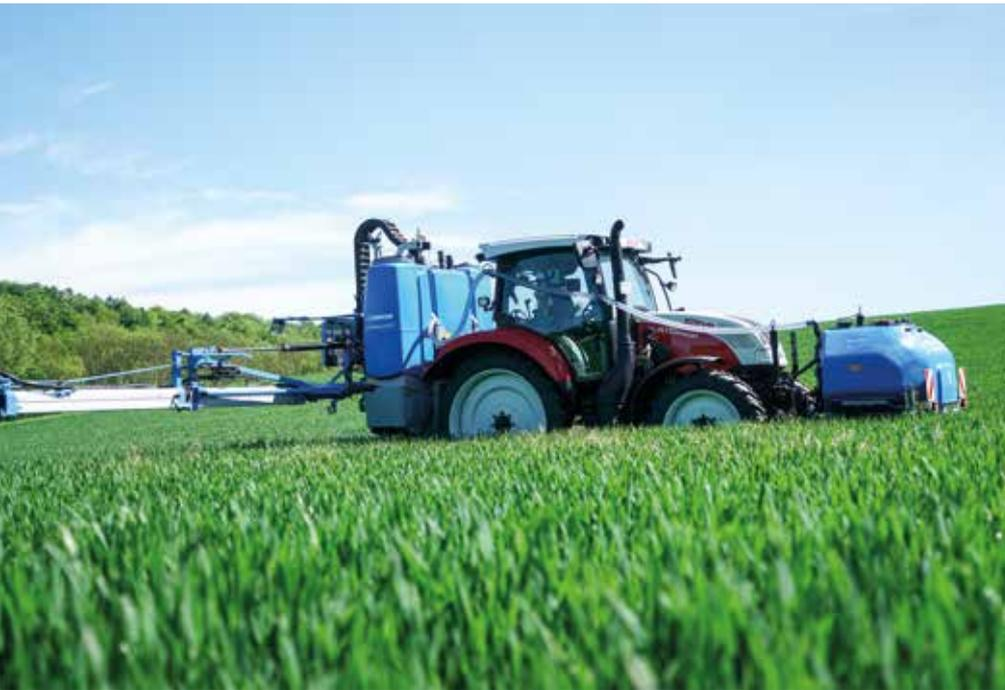
The combination of the Sirius mounted field sprayer and the Gemini front tank allows the capacity to be increased by 1,100 litres. This means not only greater acreage performance, but above all improved driver safety, as the front tank ensures balanced tractor loads.
