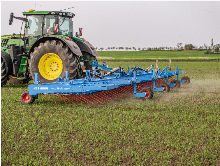
Image 2: The LEMKEN Thulit operates with constant tine pressure.
