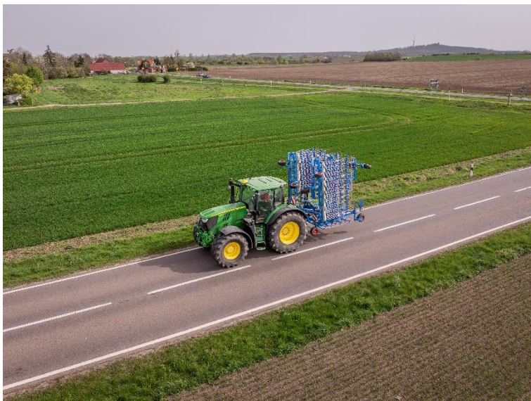
Image 3: For safe road transport, the tines on the LEMKEN Thulit are automatically folded up in addition to the five-fold folding mechanism.
