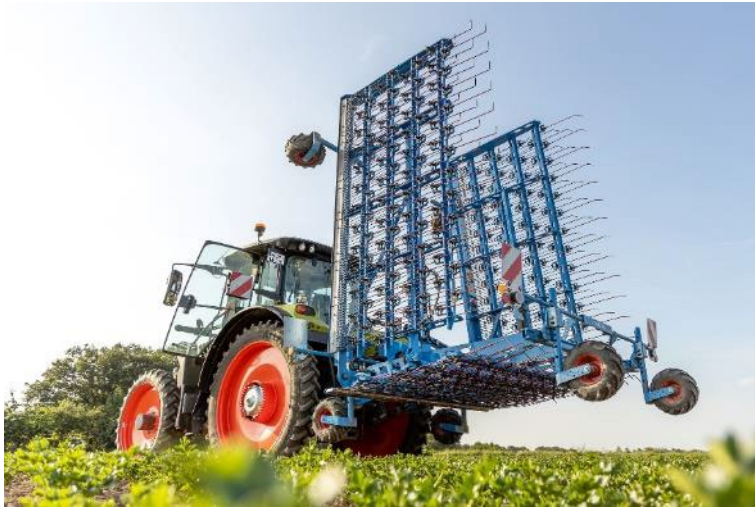
Image 3: The tines of the Thulit harrow are automatically folding for transport
