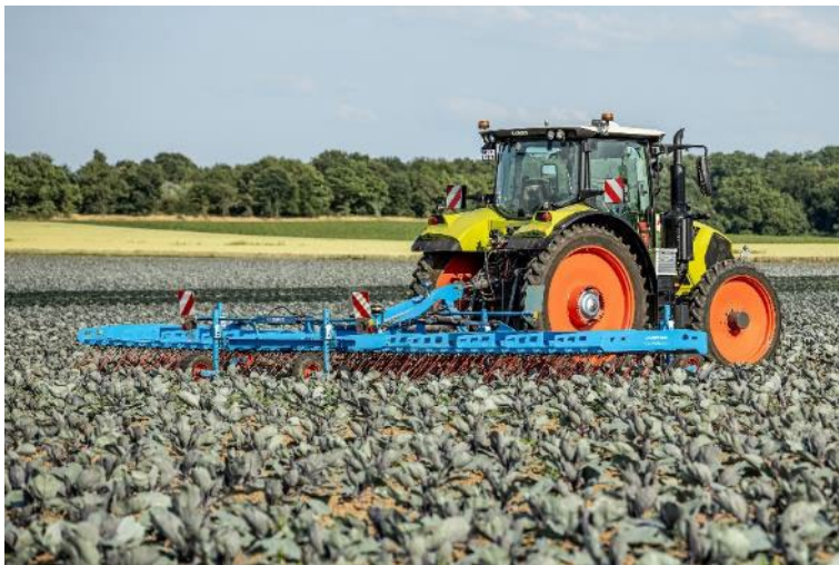
Image 2: LEMKEN harrow Thulit with four beams and eight rows of harrow tines
