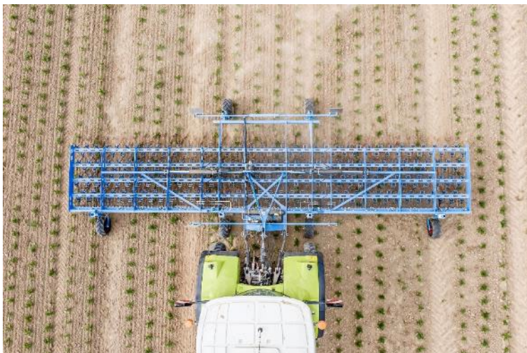
Image 2: LEMKEN harrow Thulit with four beams and eight rows of harrow tines
