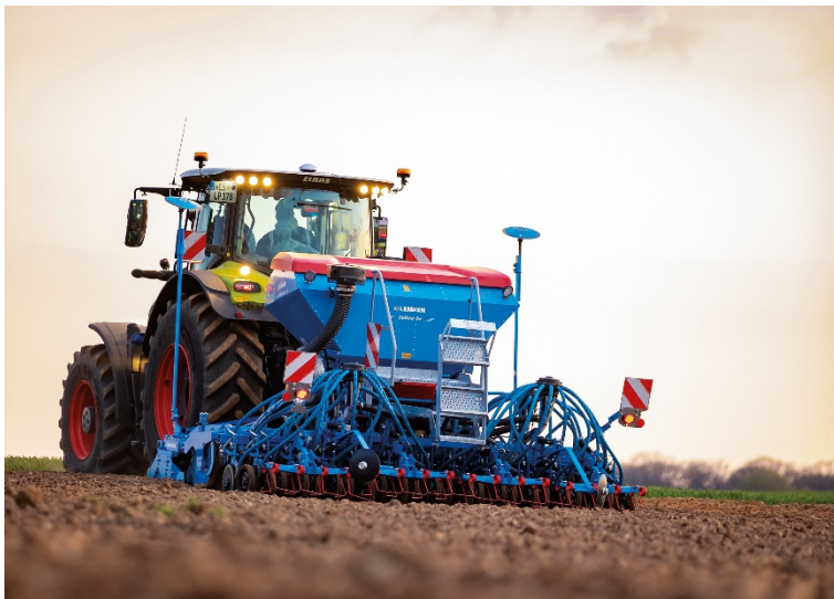
Image 1: The new Solitair 9+ Duo from LEMKEN with seed and fertiliser placement
