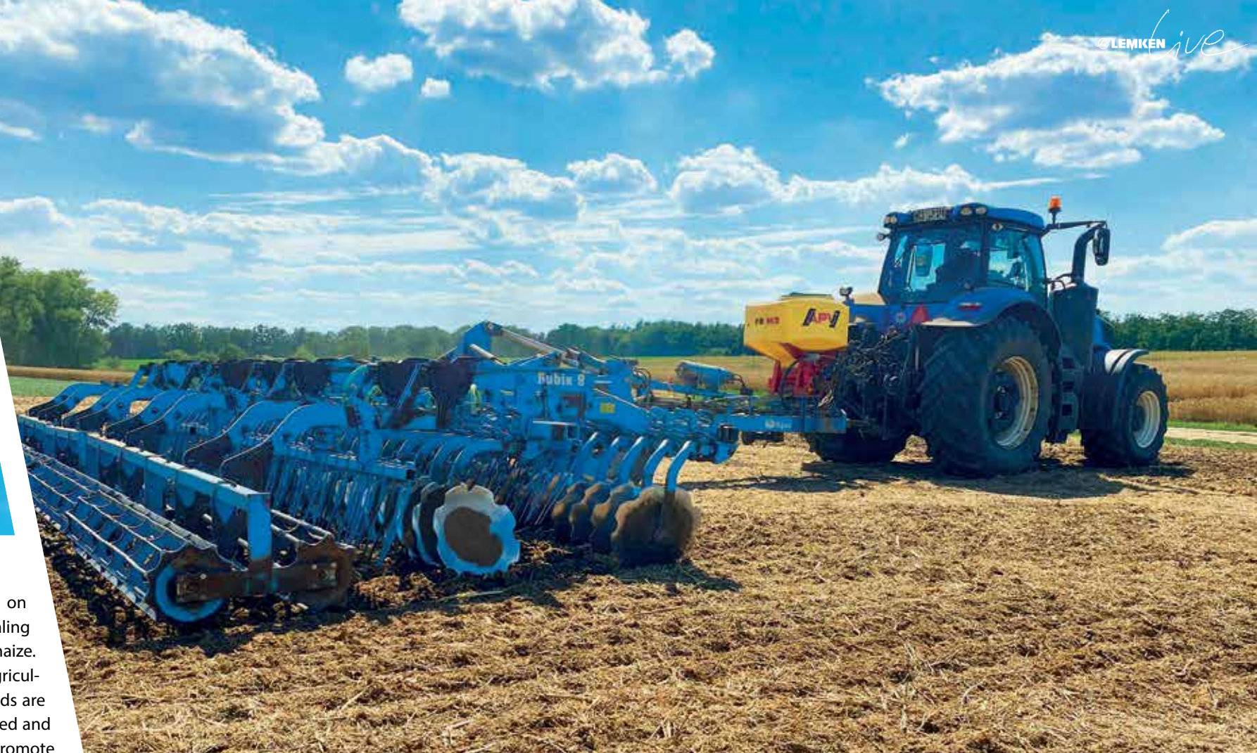
The Gigant system carrier is attached to a Rubin 9 compact disc harrow with an 8-metre working width.
