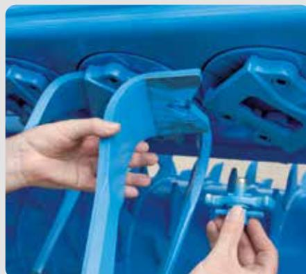
**Replacing a quick-change tine**
