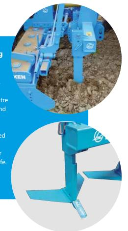
When using cultivation methods that work without ploughs, for example with mulch seed drill combinations, regularly loosening compaction in the subsoil is necessary. The Dolomit 9 pre-loosener from LEMKEN is ideal for all of these applications, and is especially suited for use with the Zirkon power harrow from LEMKEN.
