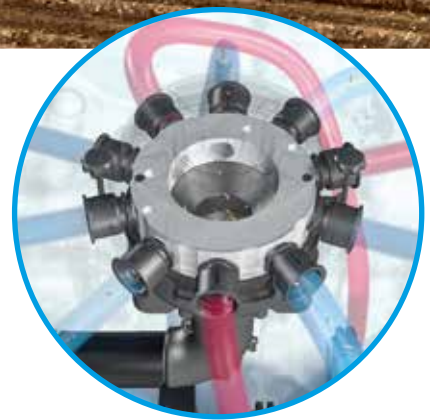
Distributor with switched tramlines
