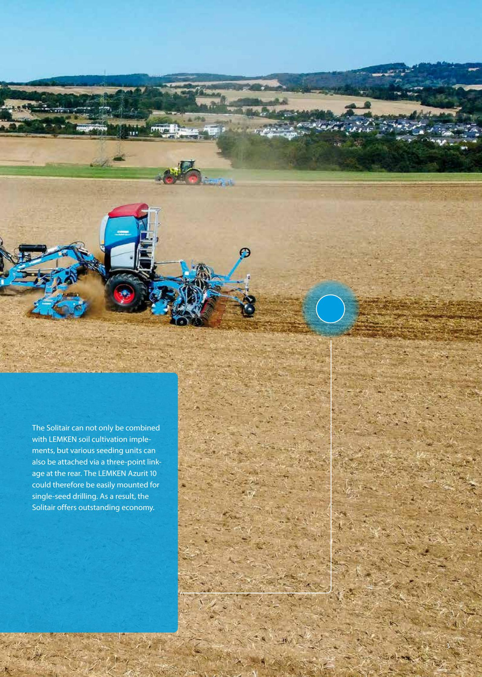
The Solitair can not only be combined with LEMKEN soil cultivation implements, but various seeding units can also be attached via a three-point linkage at the rear. The LEMKEN Azurit 10 could therefore be easily mounted for single-seed drilling. As a result, the Solitair offers outstanding economy.
