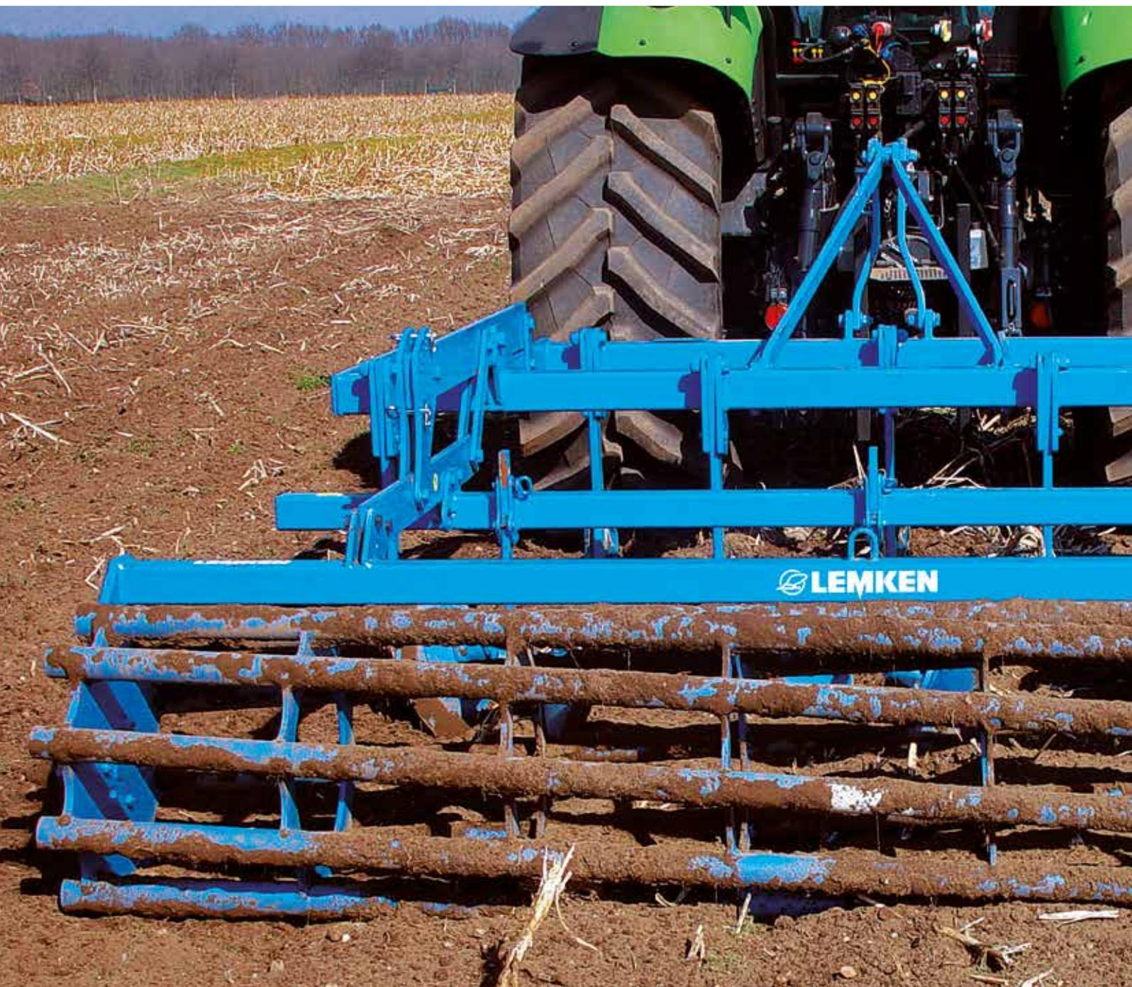
Cage rollers are available with 400 mm, 540 mm and 600 mm diameters. They represent a simple and inexpensive option for controlling the depth of implements and reconsolidating the soil. Reconsolidation is conducted in strips transverse to the direction of travel. The small diameter rollers combine excellent cultivation with low weight.
