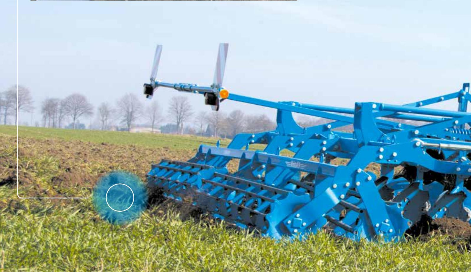
soil, the Kristall compact cultivator can be used at a depth of up to 18 cm. This medium depth cultivation tills the entire topsoil and reduces the straw concentration in the upper layer of soil - a key requirement for successful mulch sowing.
