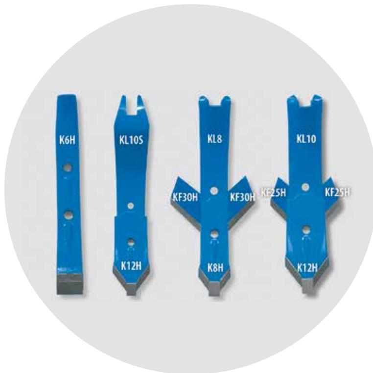
Four soldered carbide plates ensure an extremely long service life of share points. A reinforced carrier material delivers an optimal balance between carbide and steel wear. The smart use of materials on the cones and overlap sections of the share points protects the attachment bolt against wear.
