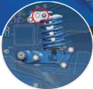
When hitting obstacles, the concave discs deflect independently upwards and rapidly return to their working position. In the basic position, the coil spring pushes the stop upwards.
