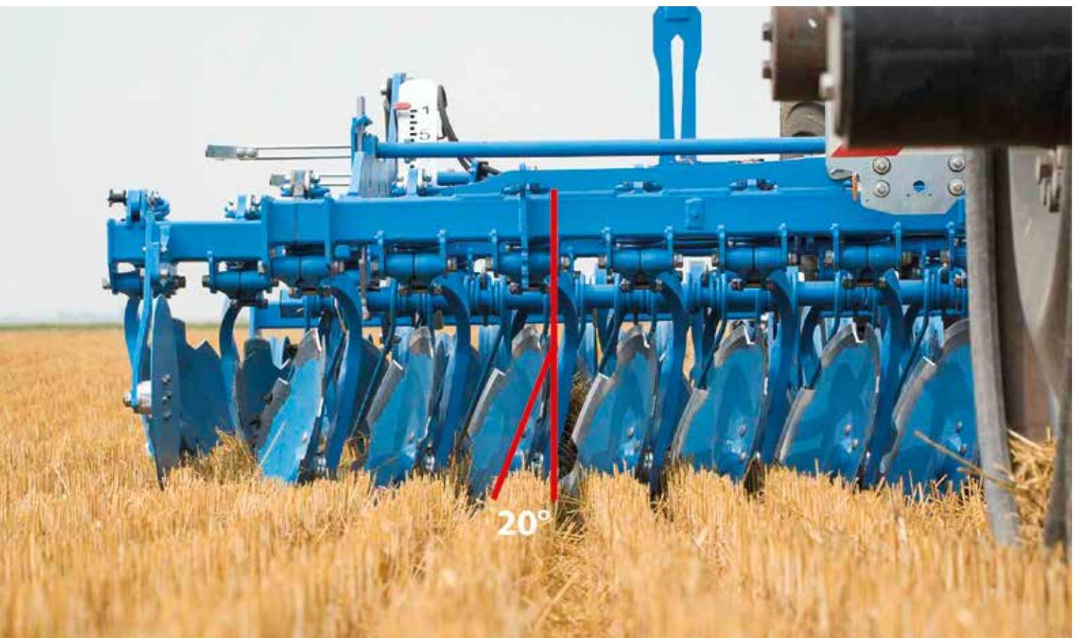
The concave discs of the **Rubin 10** are attached individually to a surface hardened stalk. Its special shape provides maximum space between the discs. The optimised clearances between the discs enable the **Rubin 10** to operate without clogging, even under very damp and sticky conditions.
