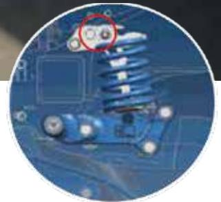
This cushions the recoil from the overload protection. The energy from the spring is transferred to the ground and does not place any strain on the frame.
