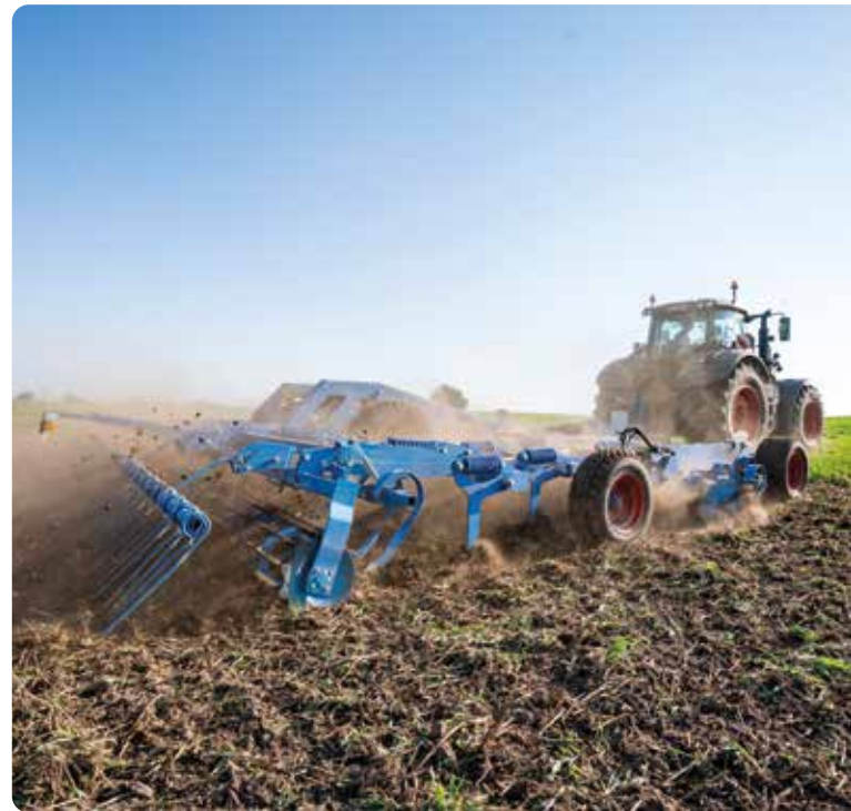
Single-row trailing harrow for use behind all rollers. This tool creates optimal germination conditions for volunteer cereals and weed seeds.
