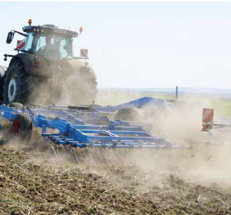
Hydraulically adjustable four-row harrow to lift plant residue and weeds towards the surface, where they'll dry and die off.
